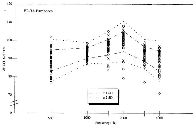
**Figure 2** Individual SPL measured near the eardrum at 500 to 4000 Hz for the ER-3A earphone ( $N = 50$ ). The "O" represents the right ear and "X" represents the left ear. Also included are  $\pm 1$  and  $\pm 2$  standard deviations (SD).
