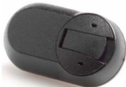
Figure 1. SAM with battery door and two microphones (Flynn, 2005).
