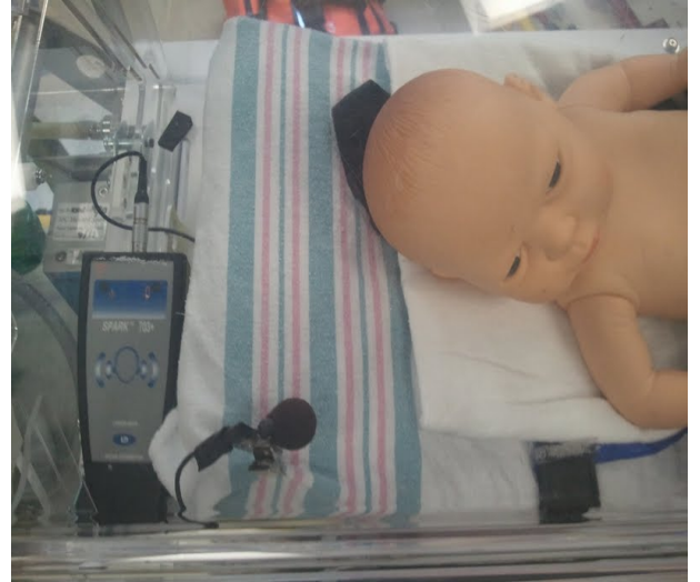
Figure 3. Noise dosimeter placed inside the infant incubator. The microphone was clipped to the upper left corner of the mattress.
