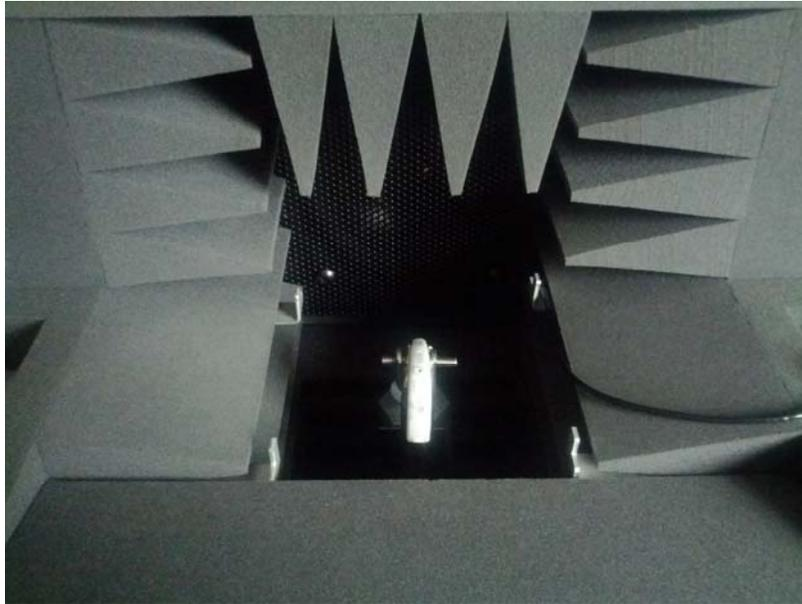
**Figure 2a: Traditional BTE hearing aid connected to an HA-2 coupler**
