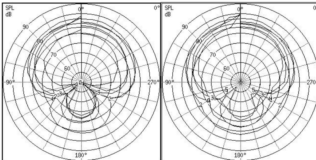
**Figure 4:** An example of a hearing aid that shows minimal change in both the FSR calculation and graphic representation of polar plots between the initial measurement (a) and the follow up measurement 3 months later (b) .
