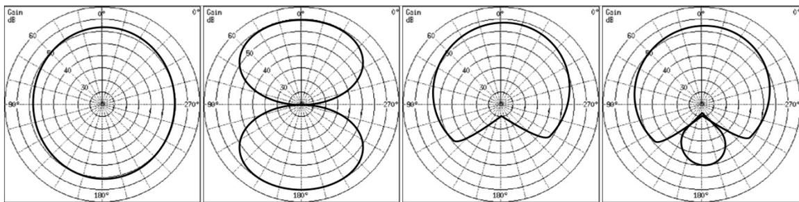
**Figure 1: Polar plots of several directional patterns are shown. From left to right: a) omnidirectional b) bi-directional c) cardioid and d) hypercardioid**
