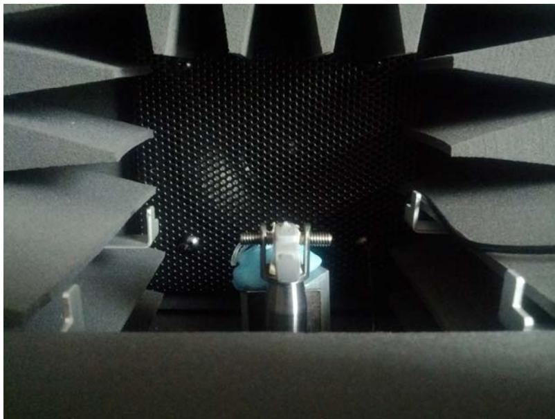
**Figure 2b: RIC BTE hearing aid connected to an HA-1 coupler**
