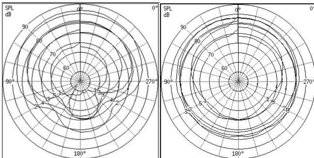
**Figure 5: An example of a hearing aid that shows remarkable change in both the FSR calculation and graphic representation of polar plots between the initial measurement (a) and the follow up measurement 3 months later (b) .**
