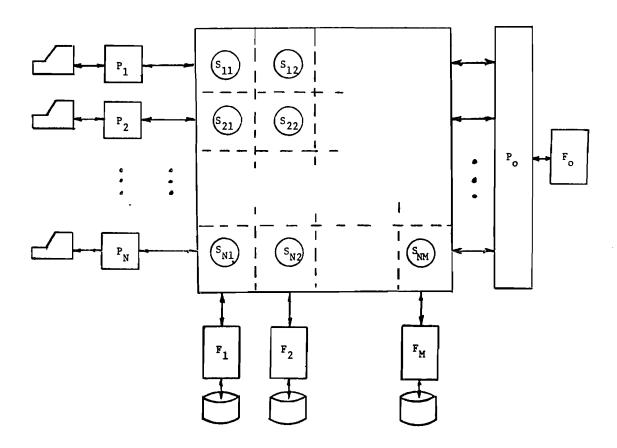
Figure 1. Block diagram of an information system based on a crosspoint switch array.
