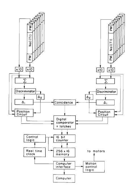
Figure 1. Block diagram of PETT-IV system electronics and interface.
