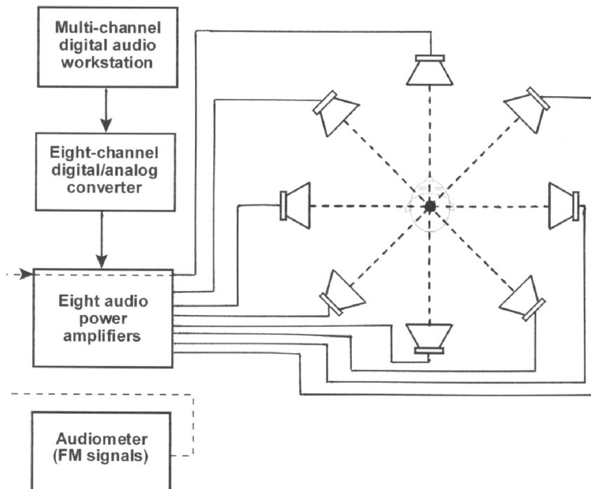
**Figure 3.** Illustration of the signal delivery and loudspeaker array used in the present study. For the 180° noise condition, only the rear loudspeaker was active. For the diffuse condition, the noise was delivered from all eight loudspeakers. For both loudspeaker conditions, the HINT sentences were delivered from the loudspeaker at 0° azimuth.
