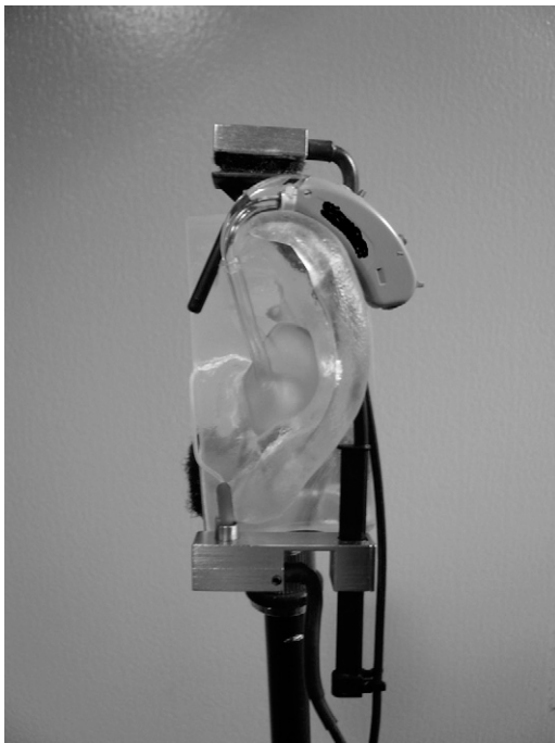
Figure 6. A sagittal view of the demonstrator ear with real-ear apparatus, custom earmold, and test hearing aid. The hearing aid is situated with front and rear hearing aid microphones oriented atop the pinna on a horizontal (level) plane. The reference microphone is placed medial to the hearing aid and adjacent to the front microphone.
