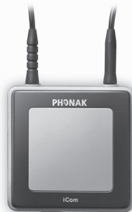
Figure 2. Illustration of the iCom Bluetooth device that was recently introduced by Phonak. This device hangs around the neck of the patient and allows for wireless communication with the hearing aids. Photo courtesy of Phonak, Inc. Used with permission.
