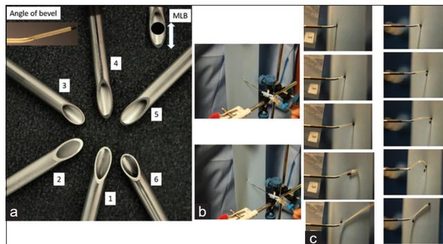
**Figure 1:** (a) Epidural needles, angulation of catheter protrusion and minimum length of the bevel (MLB). (b) The elastic band and the epidural needle are positioned such that the tip of the epidural needle and catheter touches the band. (c) Movement of the elastic band and catheter behaviour as the catheter exits the needle bevel
