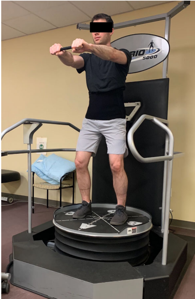
Figure 1. User undergoing dynamic postural stability testing. The multidirectional platform moves in random directions. The patient's response to these stimuli is tracked using a wearable sensor, measuring the user's center of motion in 6 planes.
