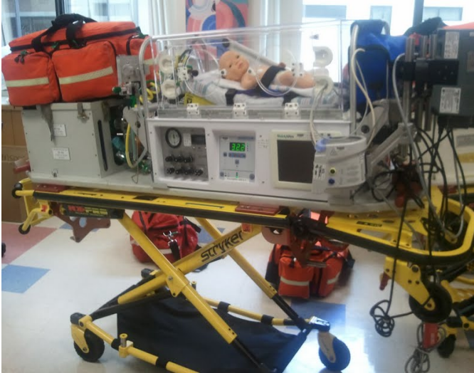
Figure 3. Noise dosimeter placed inside the infant incubator. The microphone was clipped to the upper left corner of the mattress.
