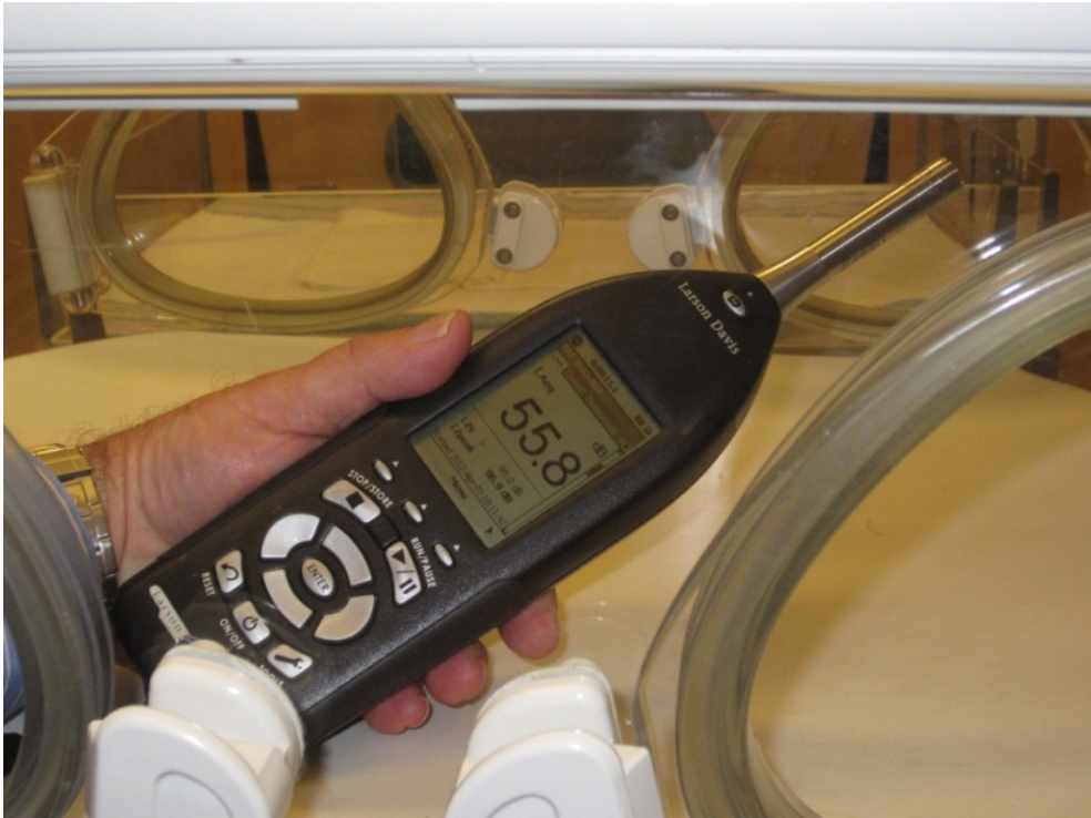
Figure 7 Larson Davis 831 Precision Sound Level Meter
