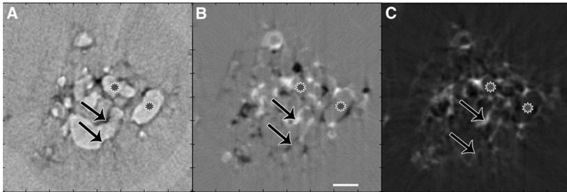
**FIG. 3.** (A) Absorption, (B) Refraction, and (C) USAXS images of a single CT slice of a PLGA scaffold in culture. Scale bar represents 450  $\mu\text{m}$ . Scaffold walls (arrows) and pores (stars) can be seen in all images. CT, computed tomography.
