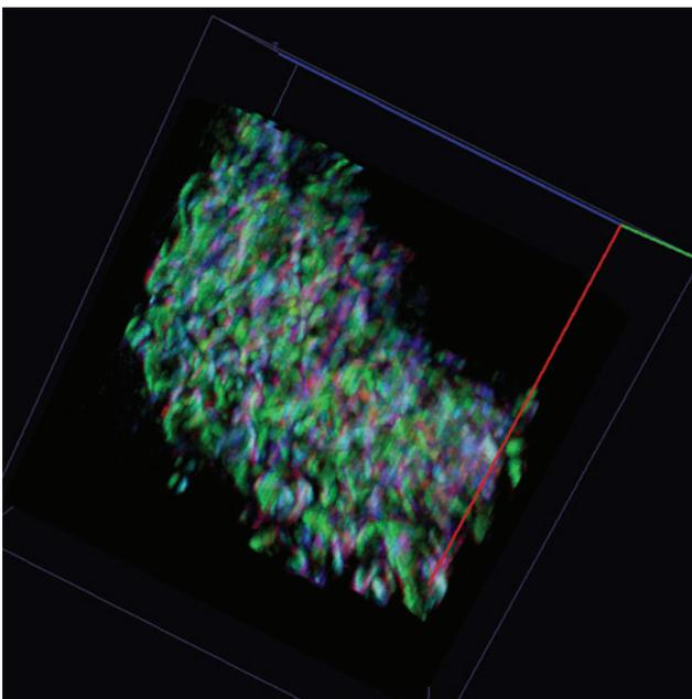
**FIG. 4.** Three-dimensional volume composite rendering of PLGA scaffold (porosity 80.9%), red represents absorption volume data, green represents refraction volume data, and blue represents USAXS volume data. These composite volumes were thresholded and used to determine porosity of the scaffolds in Table 2. Color images available online at [www.liebertpub.com/tec](http://www.liebertpub.com/tec)
