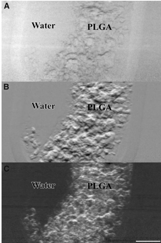
**FIG. 2.** Calculated MIR projection views: (A) Absorption, (B) Refraction, and (C) USAXS of PLGA scaffold in culture media. Scale bar represents 1 mm. MIR, multiple image radiography; PLGA, poly(lactic-co-glycolic acid); USAXS, ultra-small-angle-X-ray-scatter.
