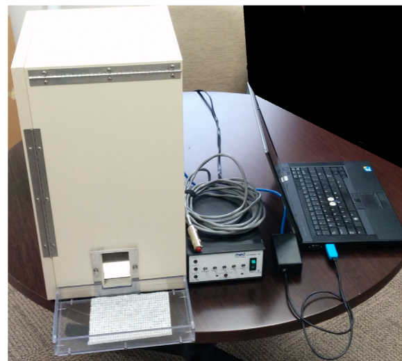
Figure 1. From left to right: Token dispenser box, Student Trainer Interface with external pushbutton, box containing relay module, connected via USB cable to laptop running TicTrainer.
