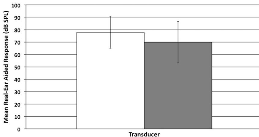
**Figure 8.** The mean REAR (in dB SPL) of 39 test hearing aids averaged across 15 discrete test frequencies when programmed to the microphone (empty bar) and t-coil (shaded bar). The error bars represent ±1 SD.
