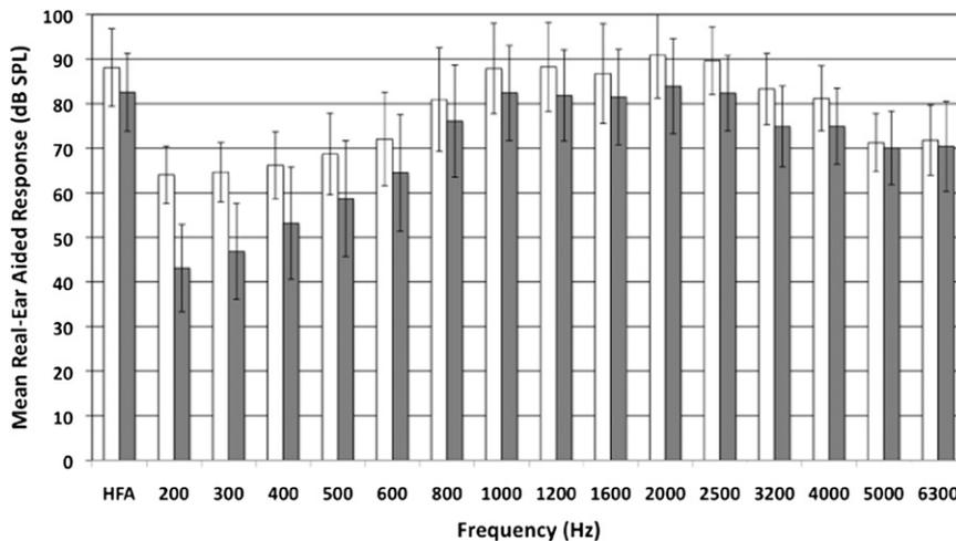
**Figure 9.** The mean REAR (in dB SPL) of the microphone (empty bars) and t-coil (shaded bars) output of 39 test hearing aids for 15 discrete test frequencies with the digispeech input signal set to 70 dB SPL. The HFA is included at the far left. The error bars represent  $\pm 1$  SD.
