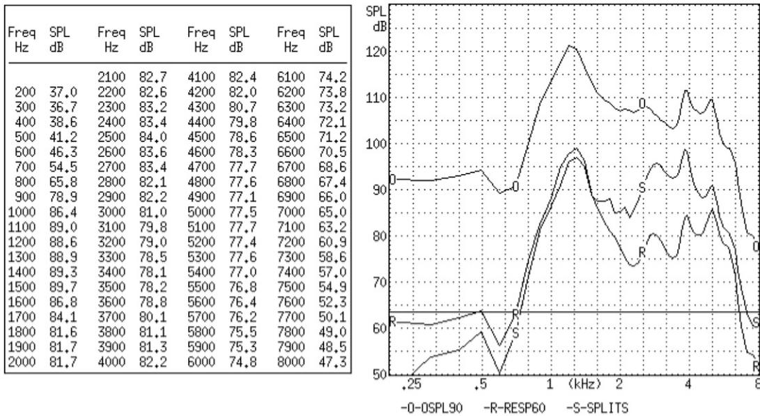
**Figure 1.** The “graphic” mode (right), which was the only viewing option available for the ANSI S3.22-2003 pure-tone coupler condition, and the “data” mode (left) available for the experimental digispeech real-ear measures condition.
