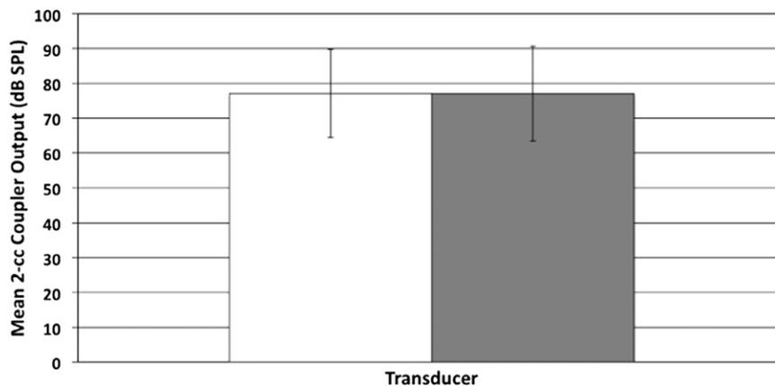
**Figure 3.** The mean coupler output (in dB SPL) of 52 test hearing aids averaged across 11 discrete test frequencies when programmed to the microphone (empty bar) and t-coil (shaded bar) using a 60 dB SPL (and 31.6 mA/M) pure-tone sweep. The error bars represent  $\pm 1$  SD.
