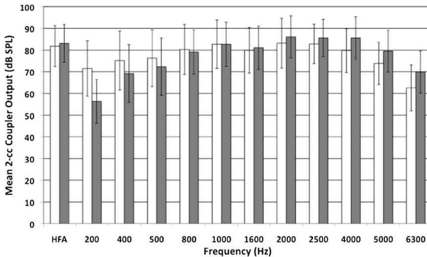
**Figure 4.** The mean coupler output (in dB SPL) of the microphone (empty bars) and t-coil (shaded bars) output of 52 test hearing aids for 11 discrete test frequencies using a 60 dB SPL (and 31.6 mA/M) pure-tone sweep. The HFA is included at the far left. The error bars represent ±1 SD.
