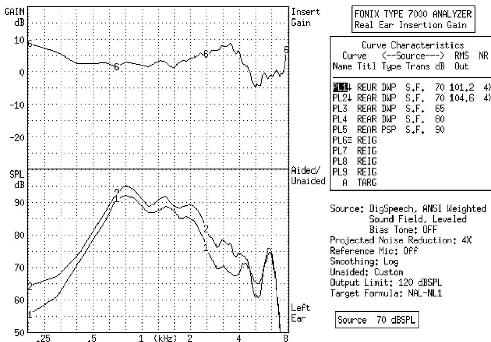
**Figure 7.** The “graphic” mode view of measured real-ear frequency responses (in dB SPL) of the programmed microphone (Curve 2) and default t-coil (Curve 1) with the digispeech input signal set to 70 dB SPL (bottom graph). The gain curve (top graph) represents the difference (in dB) between Curves 1 and 2.
