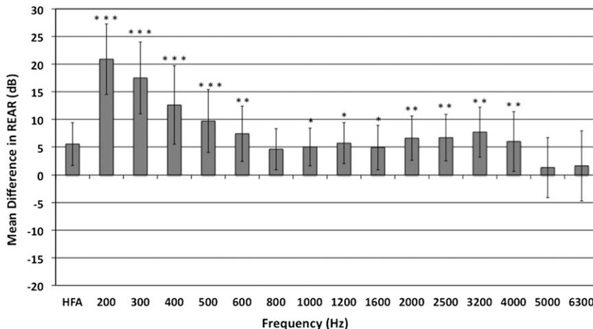
**Figure 10.** The mean difference (delta) in REAR (in dB SPL) between the microphone and t-coil output of 39 test hearing aids for 15 discrete test frequencies with the digispeech input signal set to 70 dB SPL. \*\*\* $p \leq 0.001$ ; \*\* $p \leq 0.01$ ; \* $p \leq 0.05$ . The HFA is included at the far left. The error bars represent  $\pm 1$  SD.
