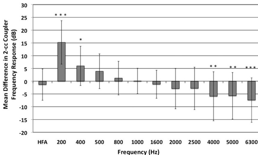
**Figure 5.** The mean difference (delta) in coupler output (in dB SPL) between the microphone and t-coil output of 52 test hearing aids for 11 discrete test frequencies using a 60 dB SPL (and 31.6 mA/M) pure-tone sweep. \*\*\* $p \leq 0.001$ ; \*\* $p \leq 0.01$ ; \* $p \leq 0.05$ . The HFA is included at the far left. The error bars represent ±1 SD.
