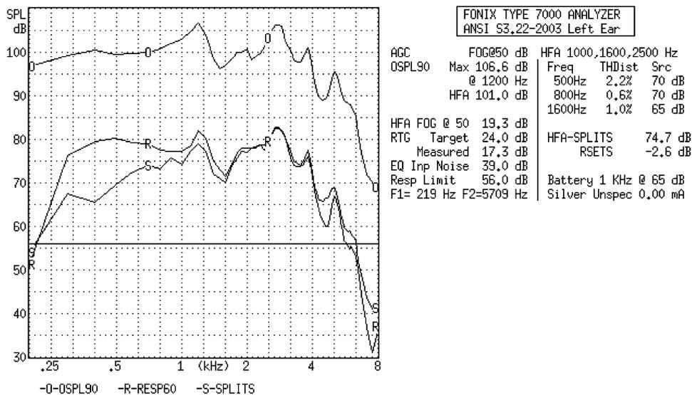
**Figure 2.** The “graphic” mode view of the measured coupler frequency responses (in dB SPL) of the programmed microphone (Curve R) and default t-coil (Curve S) to a pure-tone sweep signal via ANSI S3.22-2003. Curve 0 represents the OSPL90 microphone frequency response. Note in this case that the RSETS is  $-2.6$  dB, which means that the HFA for the t-coil is 2.6 dB lower than the HFA for the microphone.
